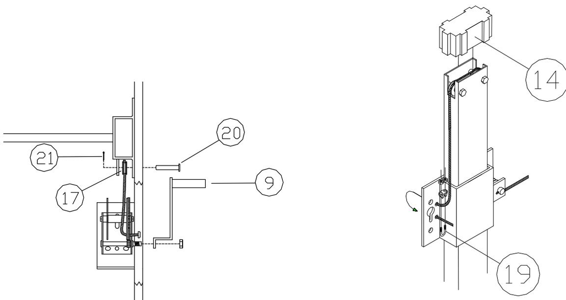
**STEP 5.** Bring top of chain (**REF. # 12**) up to the opposite side of dock, through the keyhole bracket located on the vertical lift member pocket and lock in position by sliding the chain link down the keyhole slot
