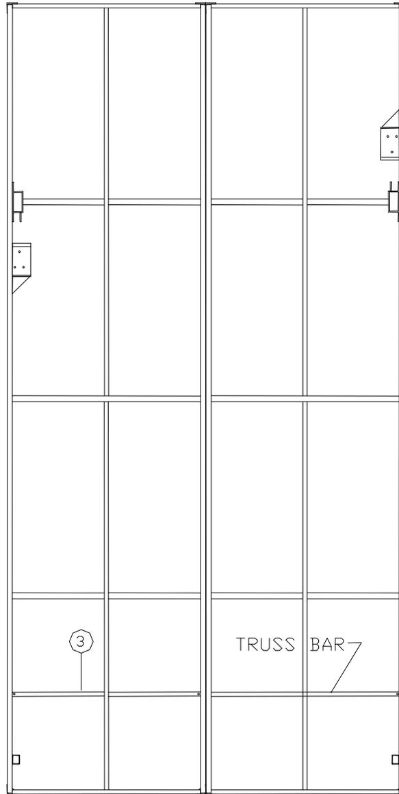
**STEP 6.** Attach the truss bars (**REF. # 3**) by placing the truss bar underneath the docks frame so that it is about 24” from shore end of the dock. Fasten truss bar to the bottom one inch square tube of the docks frame with the three J-hooks, 5/16” washers, and locknuts (**REF. # 31, 33 & 32**).
