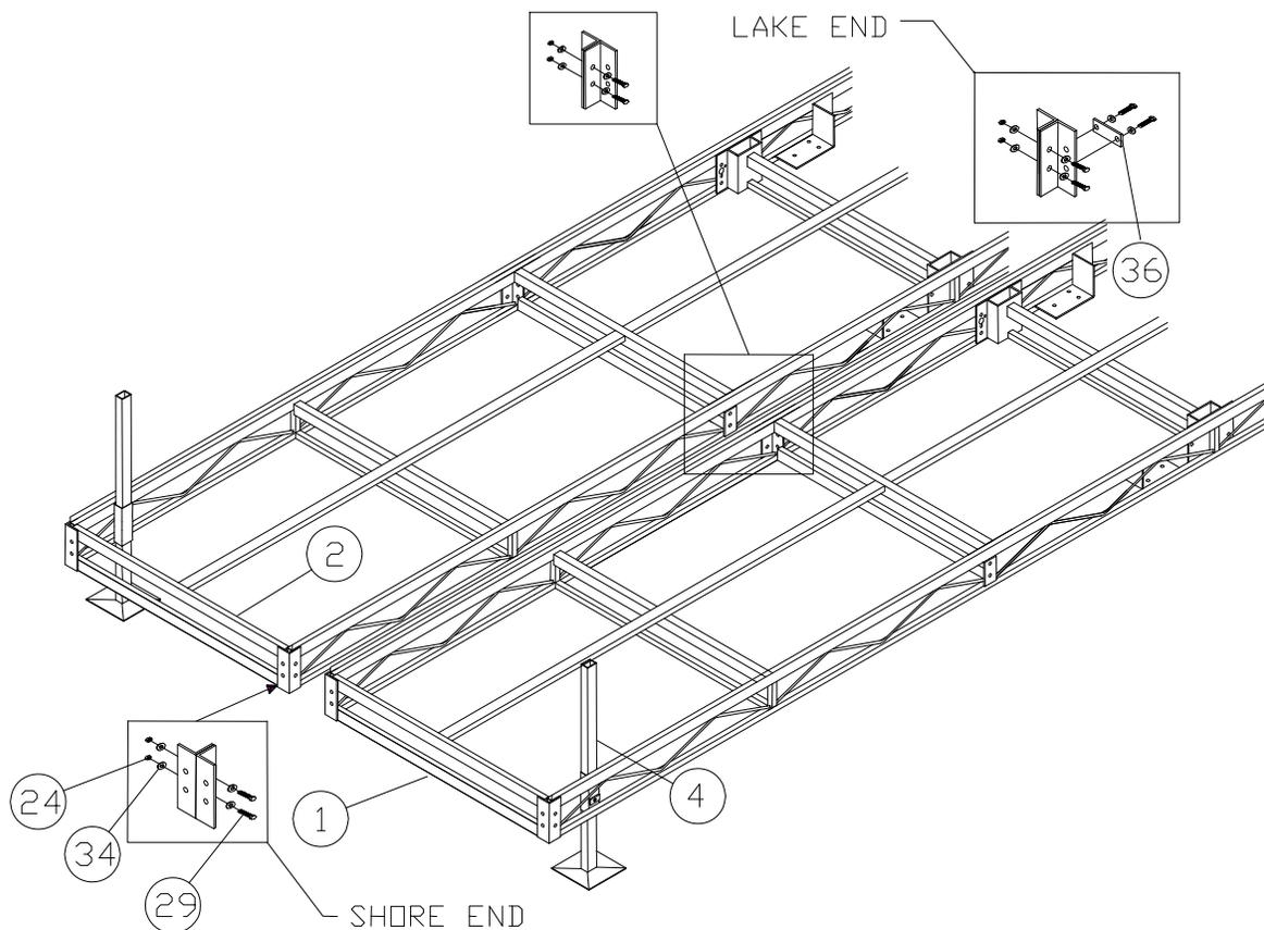
Raise the dock up approximately 30" and tighten set screws on the two posts. Support other end of dock in a safe and secure manner. Bolt winches (**REF. # 8**) to the winch plates (located to the side of the large center pockets) using 3/8 x 1" bolts & nuts.
