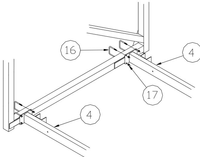
**STEP 2B.** Remove the 1/2" nuts on the 1/2" X 8" bolts (REF. # 40) that were installed in step 2 and place the center side member (REF. # 11) onto the bolts, and secure with 1/2" washers and nuts (REF. # 20 & 34). Place plastic caps (REF. # 37) on the upright and bottom end of the center side member. If not installing a canopy place the two remaining caps on the rear uprights of the outside side sections.
