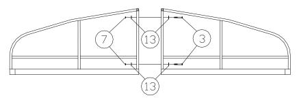
**Step 3.** Set the assembled canopy into the four mounting brackets and adjust to desired location. Place a 3/8" X 2 1/2" bolt (**REF.** # 5) through the holes in the canopy mounting bracket and secure with 3/8" washers and nut (**REF.** # 13 & 7).
